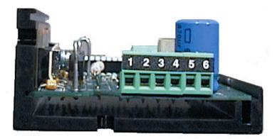
Motor And Power Supply Connector (J1)
